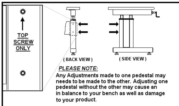
**Step 1:** With Accessories installed, crank the hand crank clockwise and between mid-point to highest point check to see if the top moves back and forth when the work surface is pushed (there will be some play, but it should be minimum)
